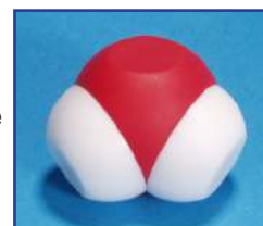
Embedded magnets are positioned at 105° from each other.
