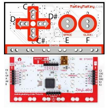
Any conductive material can be used as the input device for a computer. Because it comes preprogrammed, students with no coding experience can use it and learn to experiment with it as they start to learn coding.
